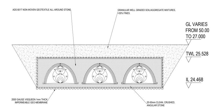
**CROSS SECTION** THROUGH ATTENUATION FACILITY SCALE 1:50
